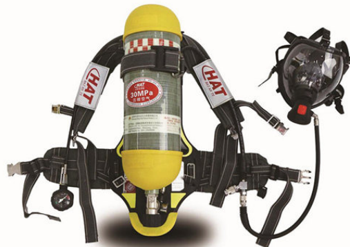
Model: RHZK6.8/A Working pressure: 30MPa Weight: ≤11KG Use time: 50±10min Cylinder volume: 6.8L
